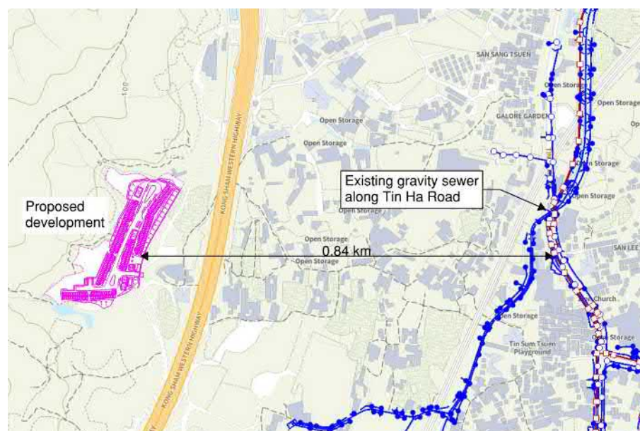
Figure 3.1 Distance between Proposed Development and Existing Sewer
